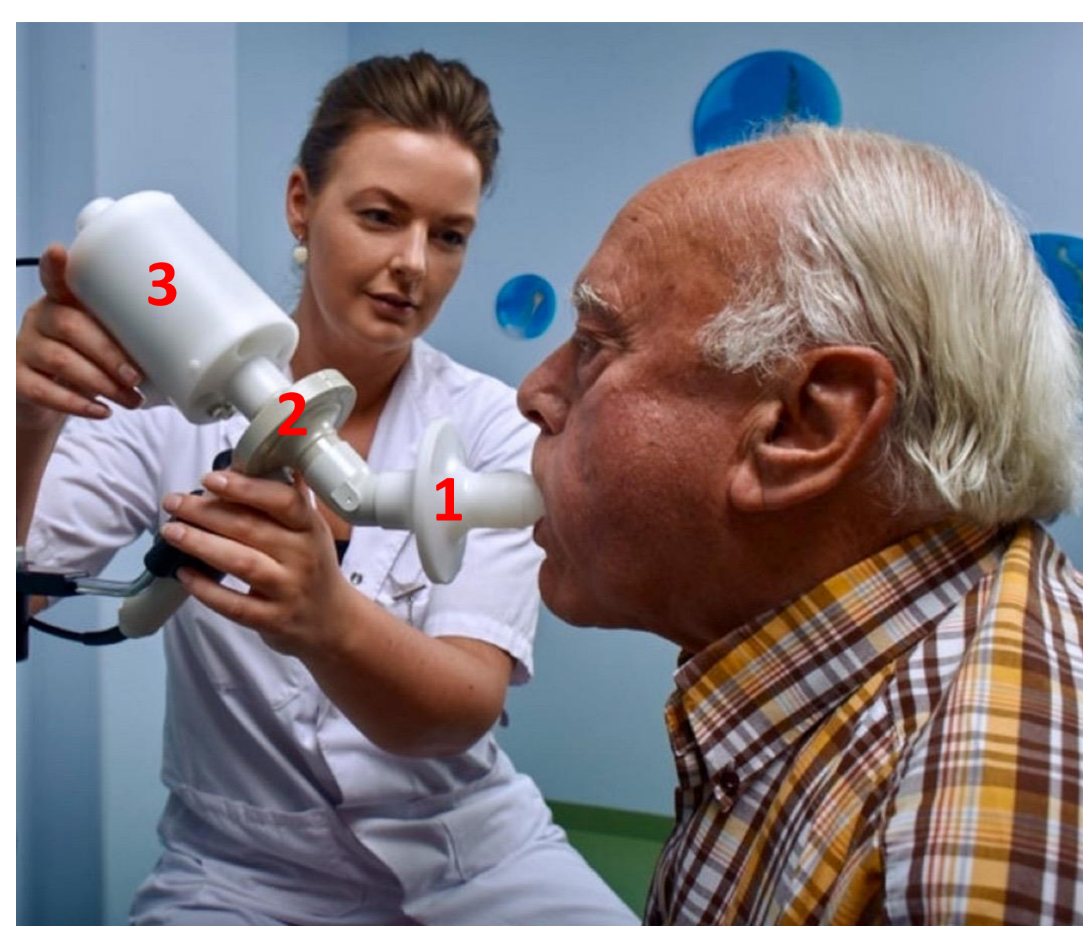
Fig 2. Frontview of the SpiroNose. → 4 identical sensor arrays monitoring exhaled breath. (De Vries J. Breath Res. 2015) → 4 reference sensor arrays monitoring ambient VOCs.
